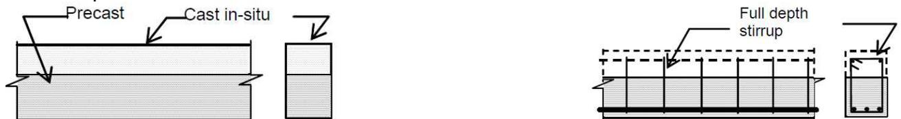
Figure 5.1-16: Composite members combining precast beams with a cast-in-place top slab.
