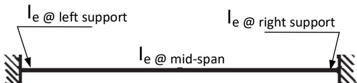
$I_e$  for Both end continuous beam =  $0.5I_e$  @ mid-span +  $0.25(I_e$  @ left support +  $I_e$  @ right support)
