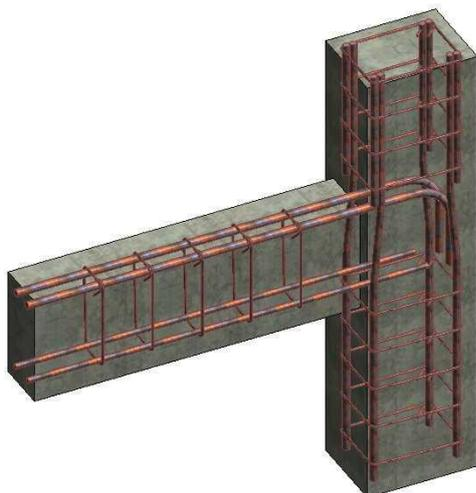
**Figure 6.4-5: Bar details at beam-column joint for bar development examples (3D Views).**
