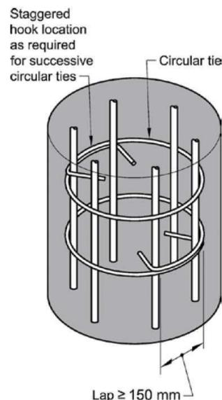
**Figure 9.2-3: Circular tie anchorage.**
