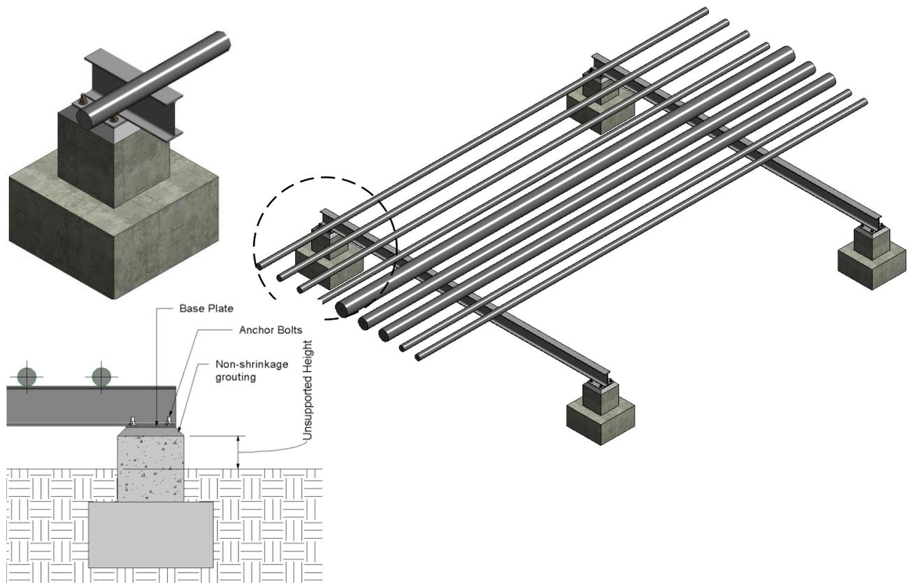
Figure 9.1-1: Pedestal used in a pipe supporting structure.
