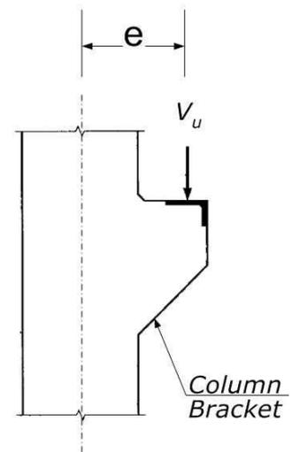
**Figure 9.5-4: Moments in columns in precast frames.**
