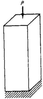
**Figure 9.1-7: Axially loaded columns.**
