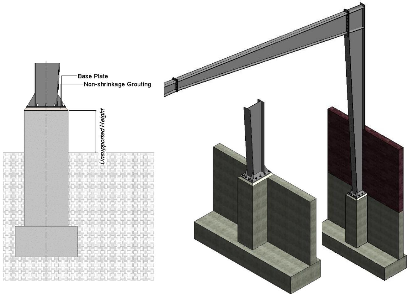
Figure 9.1-2: Pedestal used in a gable steel structure.
