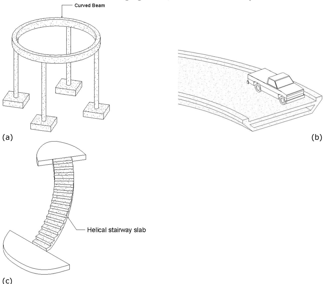
**Figure 8.1-1: Members subjected to significant torsion: (a) curved beams; (b) bridge girders; (c) helical stairway slabs.**
