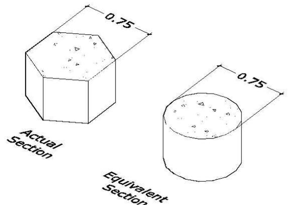
**Figure 9.4-5: Transformation of an octagonal column into the equivalent circular section.**
