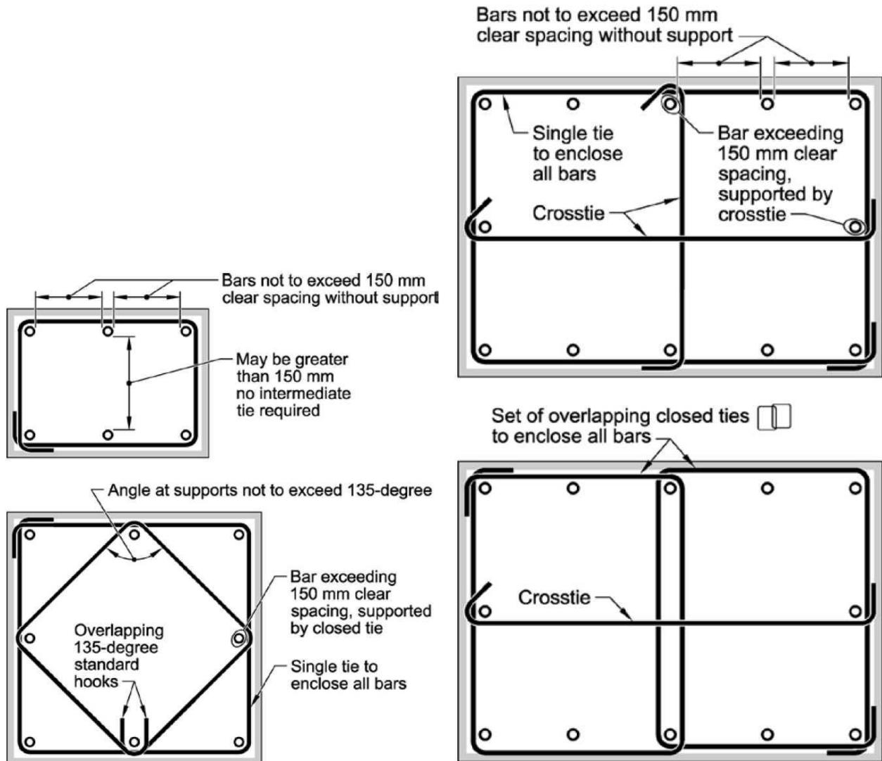
**Figure 9.2-2: Tie arrangements for square and rectangular columns.**
