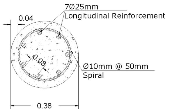
**Figure 9.2-6: Spiral column for Example 9.2-2.**
