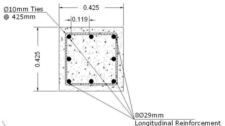
**Figure 9.3-1: Final design section for the column of Example 9.3-1.**
