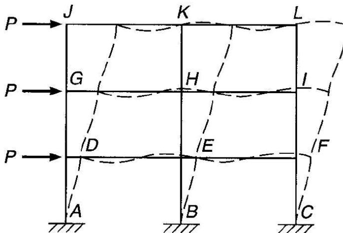
**Figure 9.5-2: Moments in columns due to lateral forces.**
