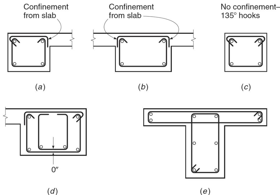
**Figure 8.2-3: Stirrup-ties and longitudinal reinforcement for torsion: (a) spandrel beam with flanges on one side; (b) interior beam; (c) isolated rectangular beam; (d) wide spandrel beam; and (e) T beam with torsional reinforcement in flanges.**
