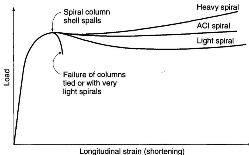
**Figure 9.2-1: Behavior of spirally reinforced and tied columns.**
