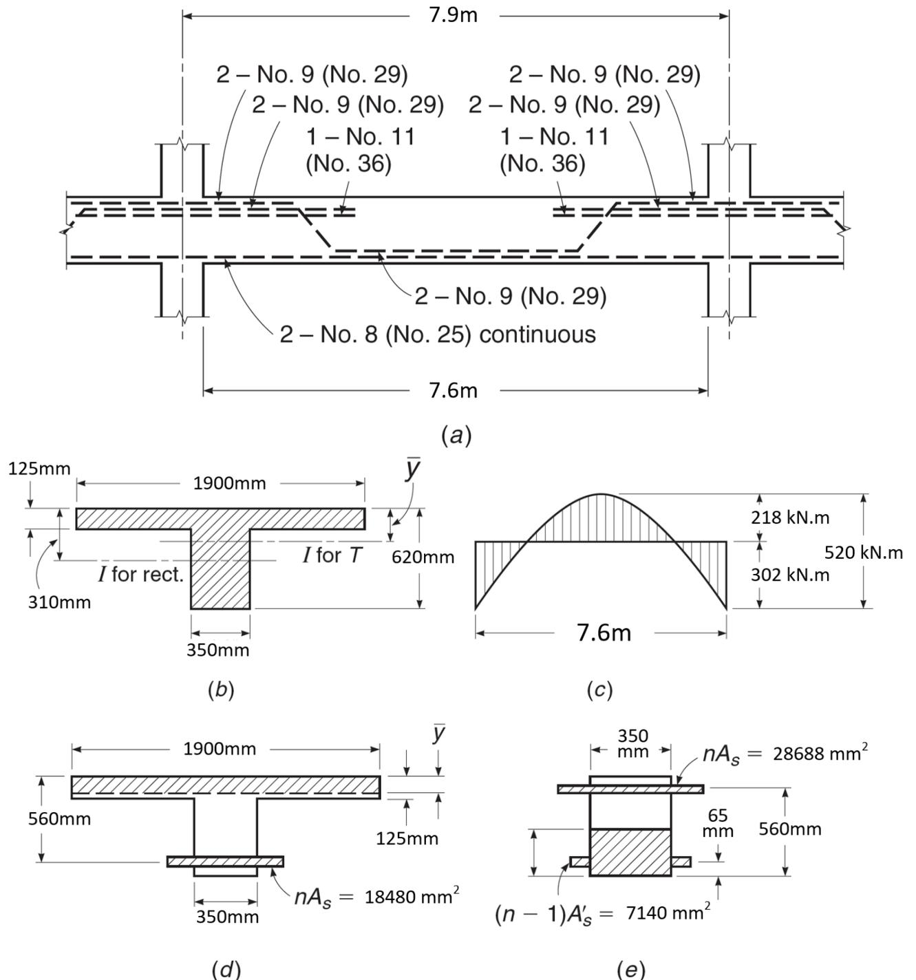
**Figure 7.7-2: Continuous T beam for deflection calculations in Example 7.7-2. The uncracked section is shown in (b), the cracked transformed section in the positive moment region is shown in (d), and the cracked transformed section in the negative moment region is shown in (e).**
