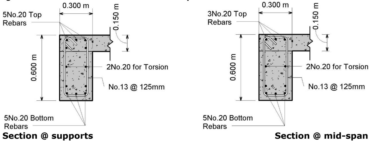
**Figure 8.3-2: Beam reinforcement for Example 8.3-1. Continue.**
