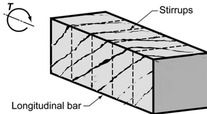
Figure 8.1-6: Reinforcement for torsion.
