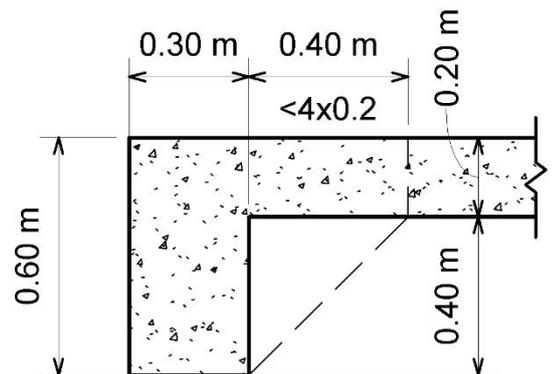
Therefore, no benefit can be obtained for torque reduction and the design should be based on  $T_u$  of 16.6 kN.m.
