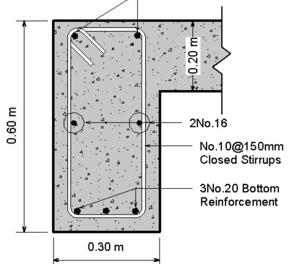
Beam Section at Supports
