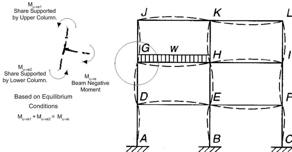
**Figure 9.5-1: Moments in columns due to frame continuity.**
