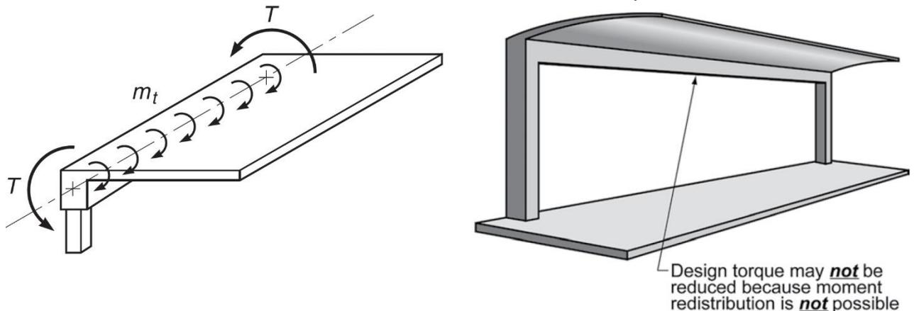
**Figure 8.1-2: Primary or equilibrium torsion at a cantilevered slab.**
