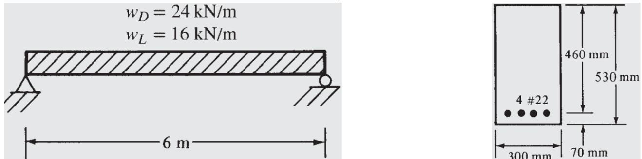
**Figure 7.7-1: Simply supported beam for Example 7.7-1.**
