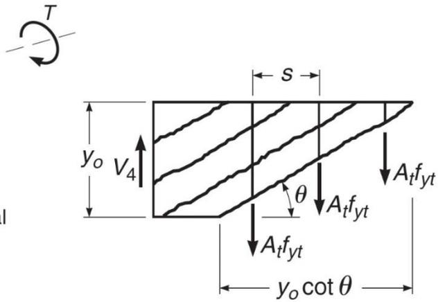
Figure 8.1-9: Vertical tension in stirrups.
