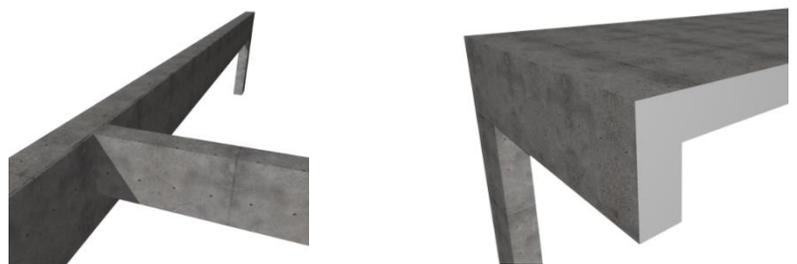
**Figure 11.8-3: Discontinuous ends with spandrel member support.**
