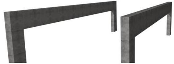
**Figure 11.8-4: Discontinuous ends with column support.**
