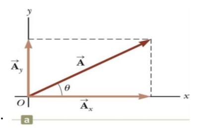
$\vec{A}_x$  and  $\vec{A}_y$  are the component vectors of  $\vec{A}$
