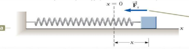
When x is positive (stretched spring), the spring force is directed to the left.
