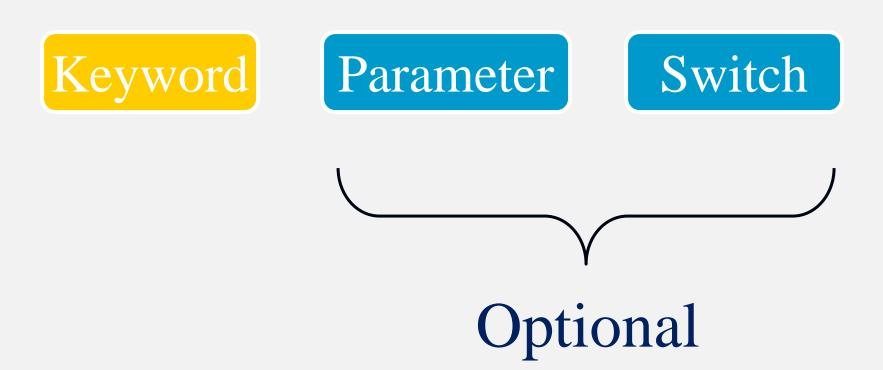
Commands are made up of one, two, or three parts as shown here. The three basic parts are called the Keyword, the Parameter, and the Switches. The last two parts are optional. One or both may not be needed with some commands.
