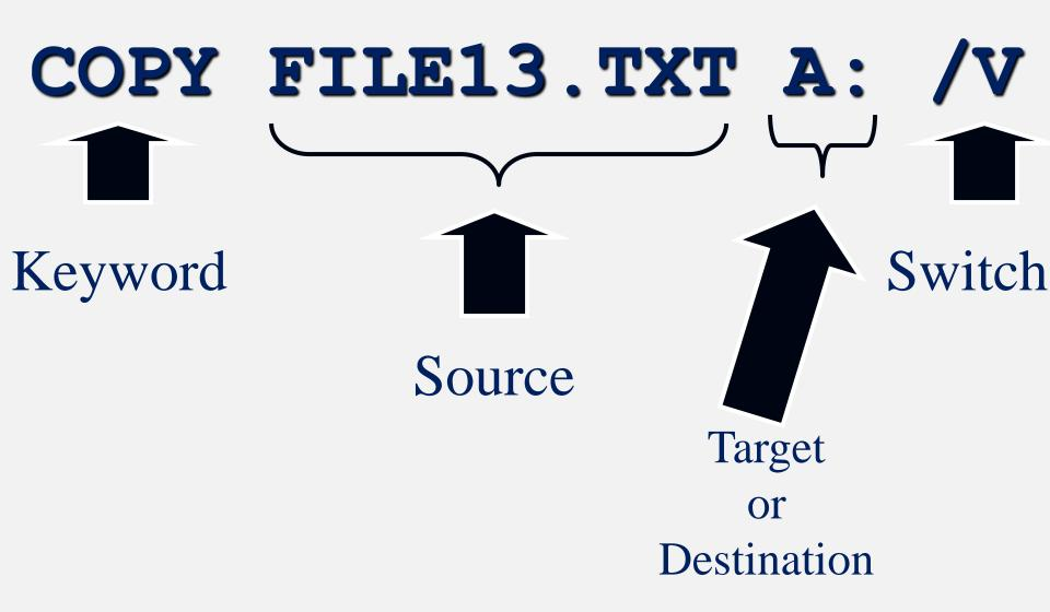
Here we see the same command but with a switch added. The  $\underline{slash V}$  at the end of the command tells the OS to verify that the copy has been recorded correctly.
