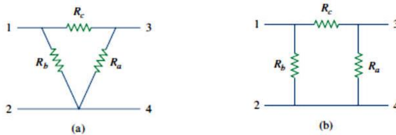
Fig 3. Two forms of the same network: (a) \Delta (b) \pi
