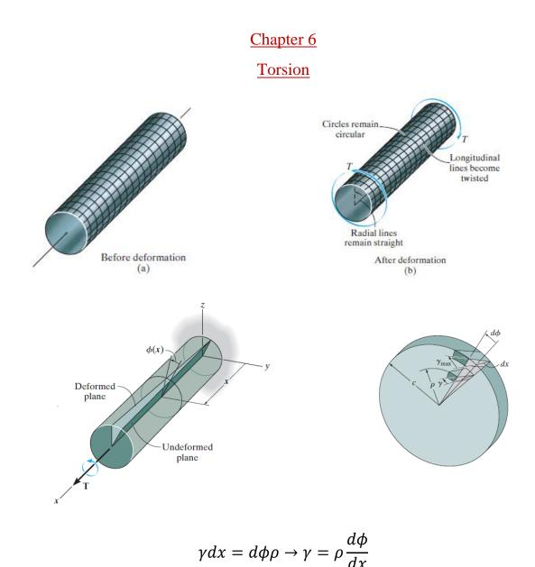
Since dx and  $d\phi$  is the same for all elements located at points on the cross section at x, then  $\frac{dx}{d\phi}$  is constant over the cross section,  $\gamma$  increases linearly with distance from the center of the axis of the shaft,
