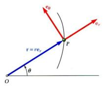
The particle velocity vector is:  $\vec{v} = \dot{r} \vec{e}_r + r \dot{\theta} \vec{e}_{\theta}$
