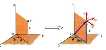
$$a_{r} = \ddot{r} - r\dot{\theta}^{2} = -0.240 \text{ m/s}^{2} - (0.481 \text{ m})(0.561 \text{ rad/s})^{2}$$
