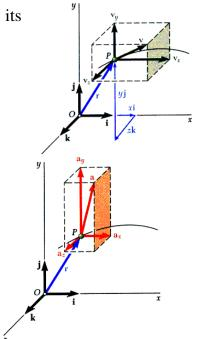
Rectangular components particularly effective when component accelerations can be integrated independently, e.g., motion of a projectile,
