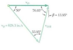
$$v_{D/B} = l\omega_{BD,...,0} = \frac{v_{D/B}}{l} = \frac{495.9 \text{ in./s}}{8 \text{ in.}} = 62.0 \text{ rad/s}$$
