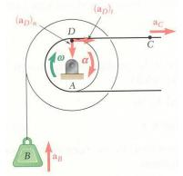
Evaluate the initial tangential and normal acceleration components of D.
