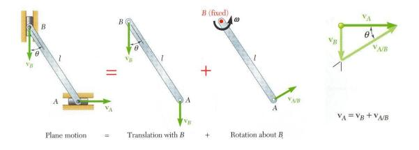
$v_{A/B}$  has the same magnitude but opposite sense of  $v_{B/A}$ . The sense of the relative velocity is dependent on the choice of reference point. Angular velocity  $\omega$  of the rod in its rotation about *B* is the same as its rotation about *A*. Angular velocity is not dependent on the choice of reference point.
