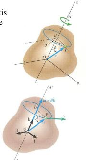
Acceleration of *P* is combination of two vectors:  $\vec{a} = \vec{\alpha} \times \vec{r} + \vec{\omega} \times \vec{\omega} \times \vec{r}$  $\vec{\alpha} \times \vec{r} =$  tangential acceleration component  $\vec{\omega} \times \vec{\omega} \times \vec{r} =$  radial acceleration component
