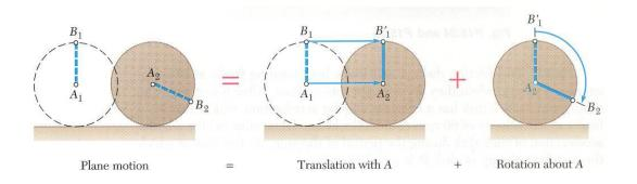
Displacement of particles A and B to  $A_2$  and  $B_2$  can be divided into two parts:
