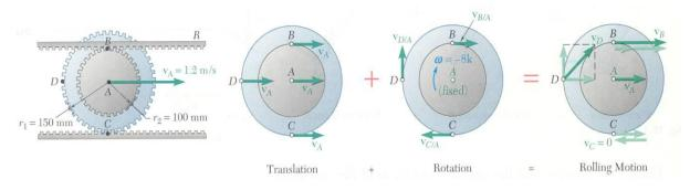
Velocity of the upper rack is equal to velocity of point B:
