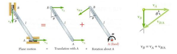
The direction of  $v_B$  and  $v_{B/A}$  are known. Complete the velocity diagram.
