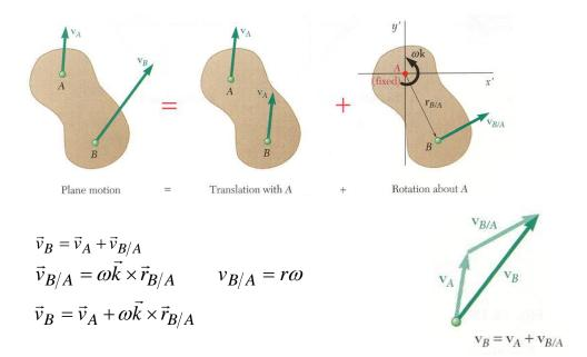
Assuming that the velocity  $v_A$  of end A is known, wish to determine the velocity  $v_B$  of end B and the angular velocity  $\omega$  in terms of  $v_A$ , l, and  $\theta$ .
