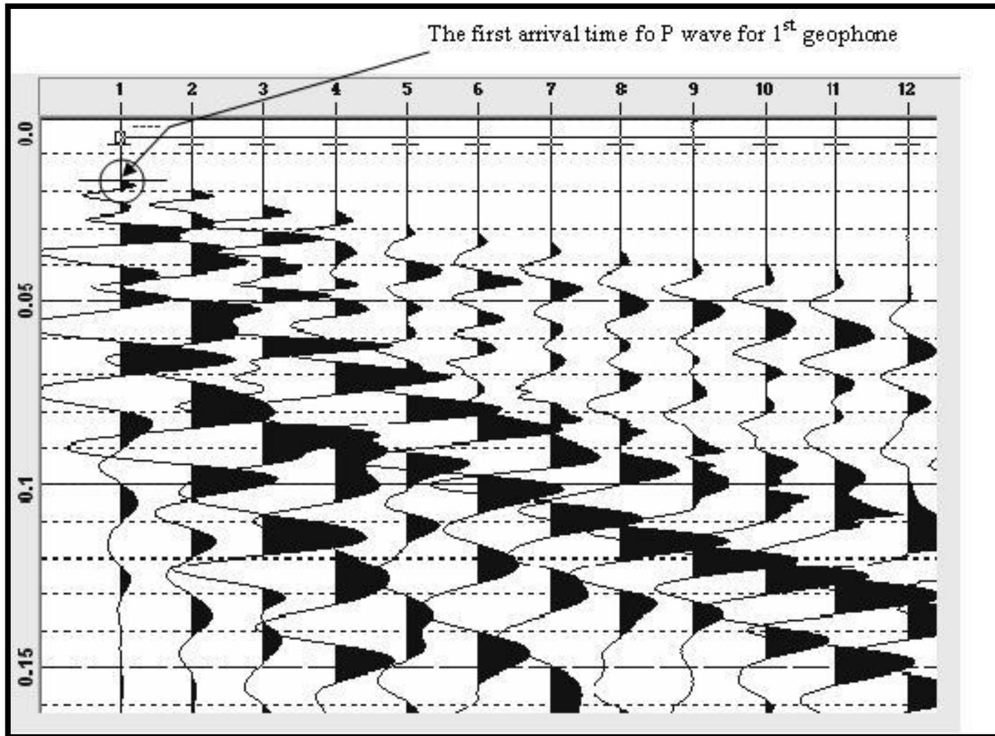
**Figure 2. Seismic refraction record.**
