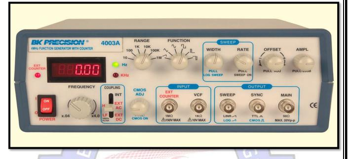
In addition to producing sine waves, function generators may typically produce other repetitive waveforms including sawtooth and triangular waveforms, square waves, and pulses. Another feature included on many function generators is the ability to add a DC offset.
