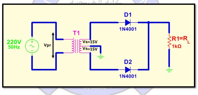
Figure 3: The Center-Tapped Full-Wave Rectifier Circuit
