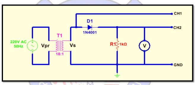
Figure 8: The Practical Half-Wave Rectifier Circuit
