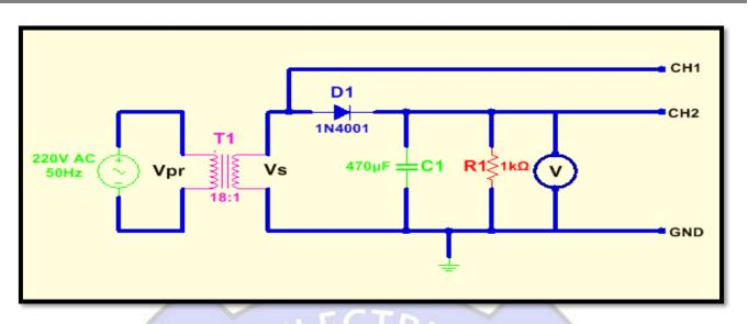
Figure 9: Practical Capacitor Filter Connected to the Half-Wave Rectifier
