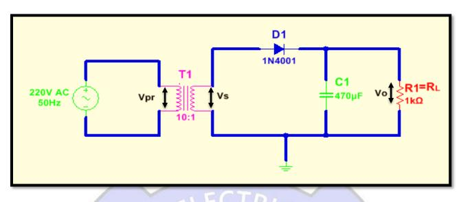
Figure 6: Half-Wave Rectifier with a Capacitor Filter
