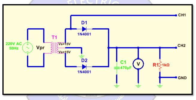
Figure 11: Practical Circuit for the Center-Tapped Full-Wave
