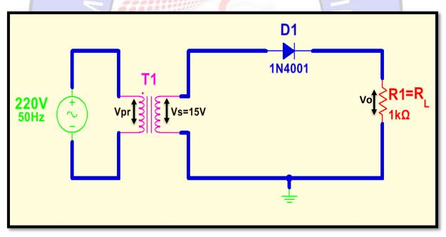
Figure 1: Half-Wave Rectifier with Transformer-Coupled Input Voltage The peak value of the secondary winding voltage  $V_{sp}$  is related to the r.m.s value by the relation:
