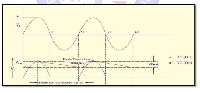
Figure 7: Output Waveform of the Capacitor Filter Connected with the Half-Wave Rectifier
