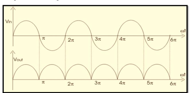
Figure 4: Waveforms of the Full-Wave Rectifier
