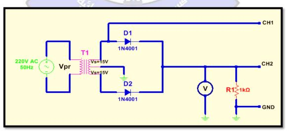
Figure 10: Practical Circuit for the Center-Tapped Full-Wave Rectifier
