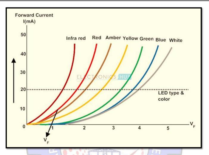
Figure 4: LED I-V Characteristics Curves Showing the Different Colors Available
