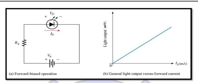
Figure 3: LED Bias Circuit and Power Output Characteristic
