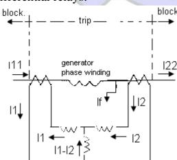
Consider the zone of protection of one phase of a generator winding shown in figure. Two current transformers are placed at the boundaries of the zone. Then for normal conditions
