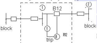
Consider  $Z_r$  is the setting impedance included in the zone. The impedance is proportional to the distance. This condition can be conveniently expressed as a requirement on the ratio of the voltage and current at the location of R12. This ratio is
