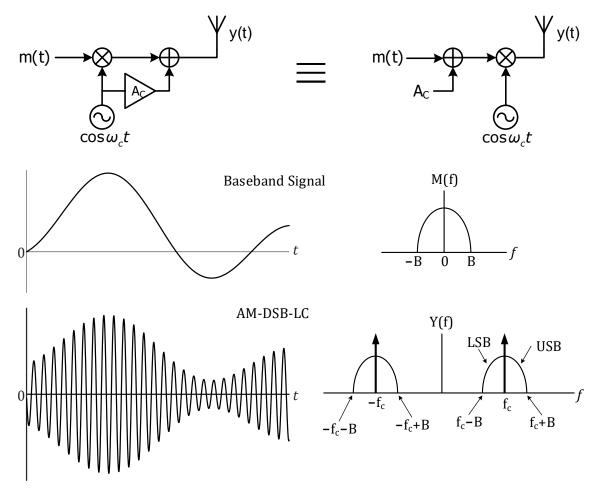
AM shifts the frequency spectrum of a signal from the zero to  $\pm f_c$  without changing its shape. Here, the bandwidth of the AM signal is double of m(t), so it is called DSB:
