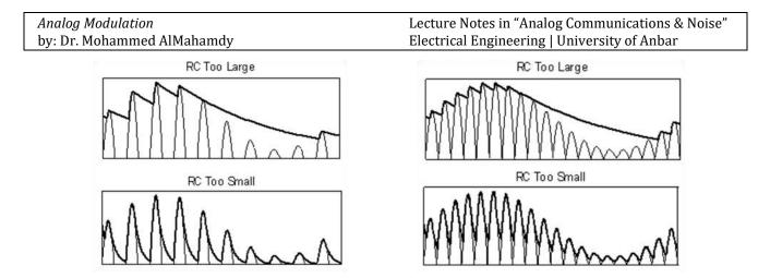
The following is an example that illustrates the asynchronous demodulation of DSB-LC.
