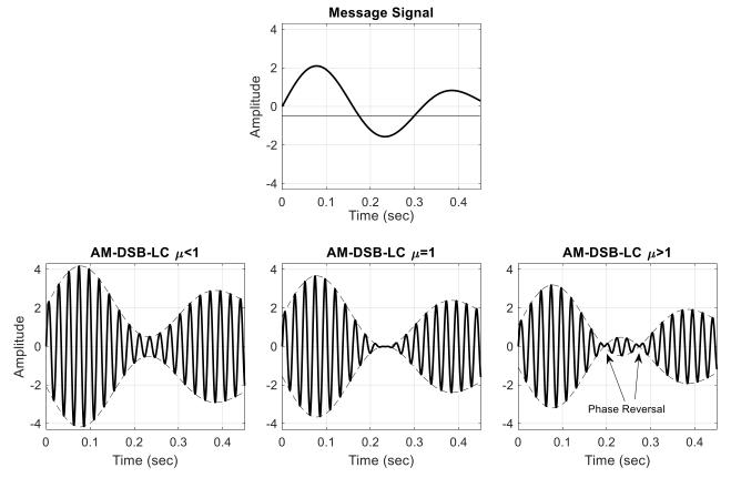
To ensure proper modulation, we must prevent the phase reversal of the modulated signal. i.e. the term  $\{1 + \mu \times m(t)\}$  must be always positive.
