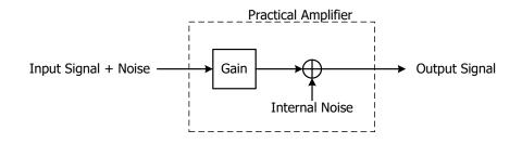
Let the received signal  $S_r$  comprise  $S_i$  as the message without noise, and  $N_i$  as the additive noise. So, if the input to the amplifier of the receiver is  $S_r = S_i + N_i$ , the output will be:
