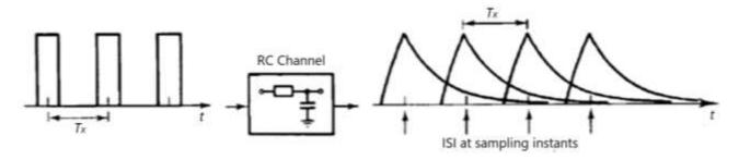
If we assume the transmission channel acts like a 1<sup>st</sup> order LPF, the response to a rectangular pulse is an exponential decay. To reduce the cross talk, the transmitted pulses must be separated by  $T_g$ . The guard time  $T_g$  is the minimum pulse spacing so that the tail of the pulse decays to a value less than  $A_{CT}$  by the time next pulse arrives.
