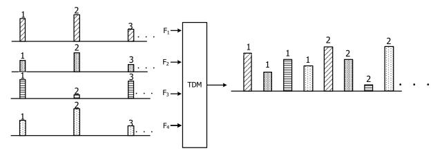
In general, we need to understand the exact design for a TDM system. In the diagram below, let  $T_x$  be the time spacing between adjacent samples in a TDM signal. If all input signals are sampled equally at  $f_s = 1/T_s$  then  $T_x = T_s/N$ , where N = number of multiplexed sampled signals. The output TDM stream frequency= clock frequency is
