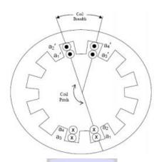
Instead of having to draw all of the slots and windings each time, we represent each distributed coil by a concentrated coil located in the center of the distribution. This is shown in Figure 5.4. The circle with a dot denotes that current is referenced out of the page while a circle with a cross indicates that current is referenced into the page. We use a, b, and c to reference the three stator phases represented in Figure.
