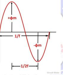
For a sinusoidal wave the r.m.s or effective value is 1.11 times the average value. r.m.s value of e.m.f induced /turn =1.11 × 4  $f \phi_m$
