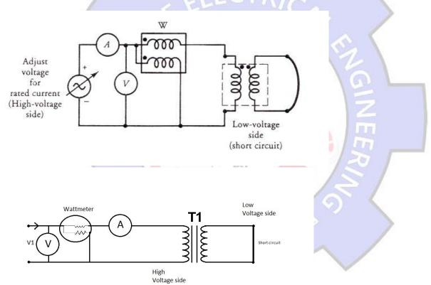
If Vsc is the voltage required to circulate rated load current, then:
