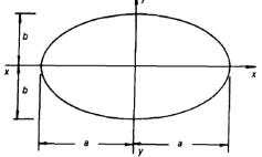
To satisfy the B.C. and  $\frac{\partial^2 \phi}{\partial x^2} + \frac{\partial^2 \phi}{\partial y^2} = F$  the stress function taking as:
