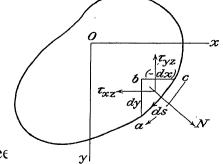
For the lateral surface of the bar, which is free has normal perpendicular to the *z*-axis, we have
