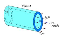
\*The hoop stress is the force exerted circumferentially (perpendicular both to the axis and to the radius of the object) in both directions on every particle in the cylinder wall.
