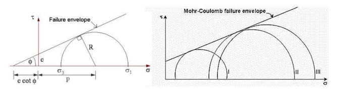
Where  $\tau_f$  = shear stress on the failure plane c = apparent cohesion
