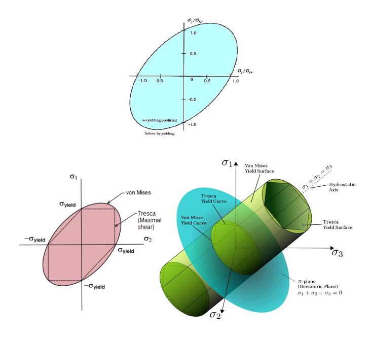
\* Distortion is the deformation from shearing stresses, deviator stresses causes change in angles and no change in volume.
