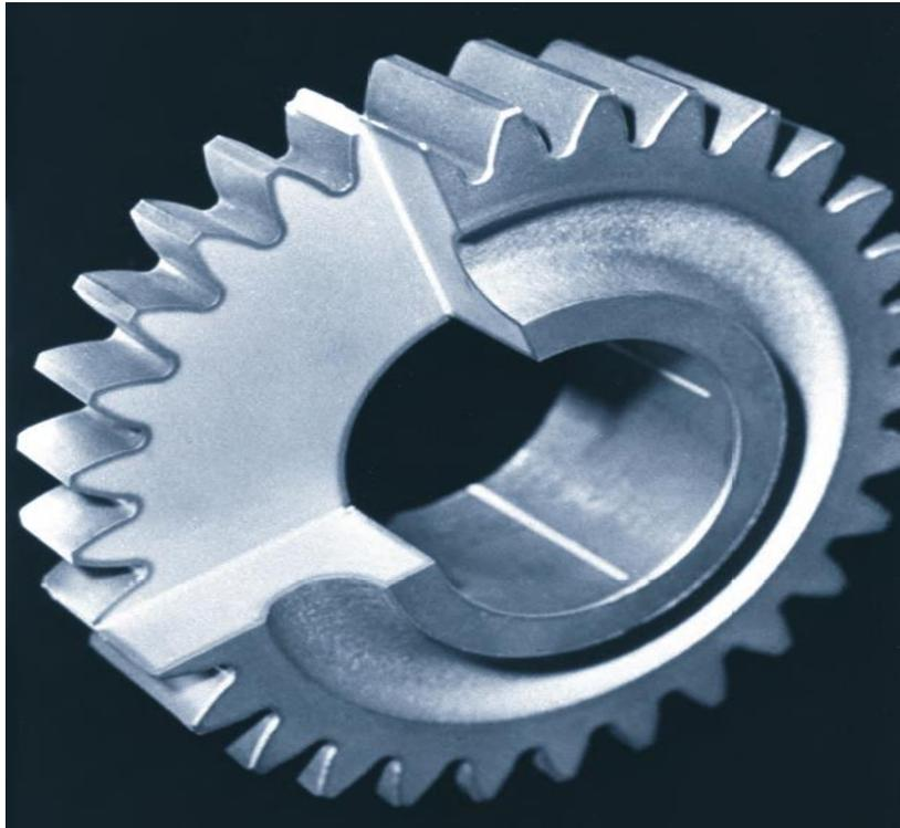
Photograph of a steel gear that has been “case hardened.” The outer surface layer was selectively hardened by a high-temperature heat treatment during which carbon from the surrounding atmosphere diffused into the surface. The “case” appears as the dark outer rim of that segment of the gear that has been sectioned. Actual size.
