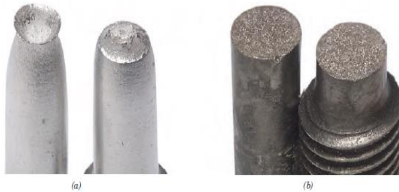
Figure 4-4 (a) Cup-and-cone fracture in aluminum. (b) Brittle fracture in a mild steel.
