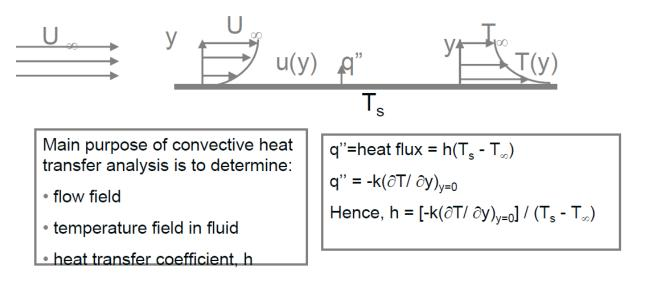
The expression shows that in order to determine h, we must first determine the temperature distribution in the thin fluid layer that coats the wall.
