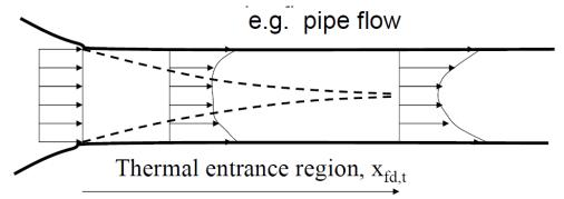
For laminar flows the thermal entrance length is a function of the Reynolds number and the Prandtl number:  $x_{fd,t}/D \approx 0.05 Re_D Pr$ , where the Prandtl number is defined as  $Pr = v/\alpha$  and  $\alpha$  is the thermal diffusitivity.
