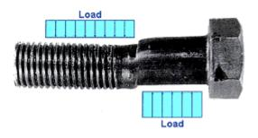
Shear stress is never uniformly distributed, but this equation can be used when dealing with small areas such as the area of a bolt or rivet.
