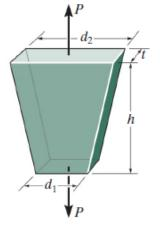
**<u>O</u> 3**: Determine the relative displacement of one end of the tapered plate with respect to the other end when it is subjected to an axial load P.
