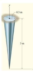
**Example 4:** A member is made of a material that has a specific weight of  $\gamma = 6 \text{ kN/m}^3$  and modulus of elasticity of 9 GPa. If it is in the form of a *cone* having the dimensions shown in Figure, determine how far its end is displaced due to gravity when it is suspended in the vertical position.
