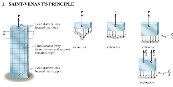
The *localized deformation* caused by *P* vanishes at a location sufficiently away (at least equal to the *largest dimension* of the loaded cross section) from the point of application of the load.
