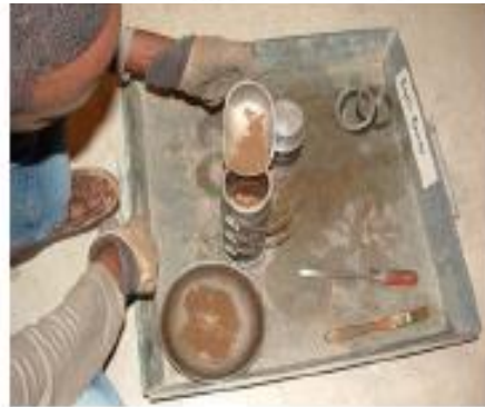
(c) Filling mold with one soil layer
