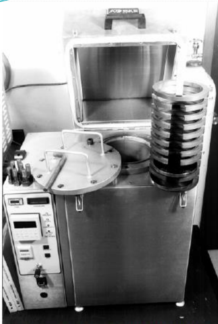
Pressure Vessel Built into Oven
