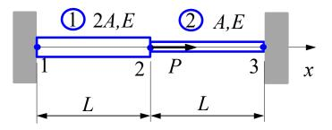
*Problem*: Find the stresses in the two bar assembly which is loaded with force *P*, and constrained at the two ends, as shown in the figure.
