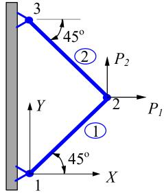
This simple structure is used here to demonstrate the assembly and solution process using the bar element in 2-D space.
