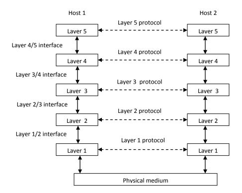
The entities comprising the corresponding layers on different machines are called peers. The peers may be processes, hardware, devices, or even human being. In the words, it is the peers that communicate by using the protocol.
