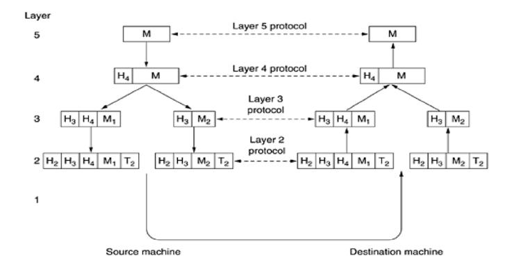
Always there is limit to the size of messages transmitted by layer 3, so layer 3 must break incoming messages into smaller units, packets, prep ending a layer 3 header to each packet. At the receiving machine the messages moves upward from layer to layer with headers being stripped off as it progresses. None of the headers for layers below n are passed up to layer n.
