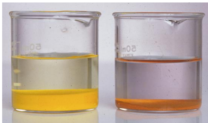
Figure 13.5 Two precipitates of \text{PbCrO}_4 . In Beaker A, combining 0.1 M \text{Pb}(\text{NO}_3)_2 and 0.1 M \text{K}_2\text{CrO}_4 forms the precipitate under conditions of high RSS . The precipitate forms rapidly and consists of very small particles. In Beaker B, heating a solution of 0.1 M \text{Pb}(\text{NO}_3)_2 , 0.1 M \text{Cr}(\text{NO}_3)_3 , and 0.1 M \text{KBrO}_3 slowly oxidizes \text{Cr}^{3+} to \text{CrO}_4^{2-} , precipitating \text{PbCrO}_4 under conditions of low RSS . The precipitate forms slowly and consists of much larger particles.
