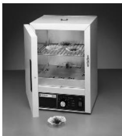
Conventional laboratory oven used for drying materials.
