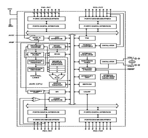
Pinouts & Modules of ATMega microcontroller ATmega8535/16/32 bobuino pinout
