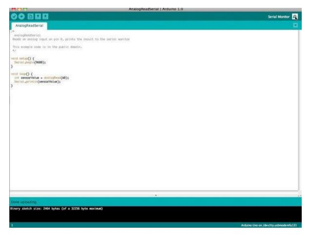
The serial monitor allows your computer to connect serially with the Arduino. This is important because it takes data that your Arduino is receiving from sensors and other devices and displays it in real-time on your computer. Having this ability is invaluable to debug your code and understand what number values the chip is actually receiving.
