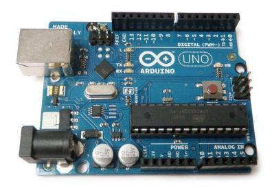
An Arduino is an open-source microcontroller development board. In plain English, you can use the Arduino to read sensors and control things like motors and lights. This allows you to upload programs to this board which can then interact with things in the real world. With this, you can make devices which respond and react to the world at large.
