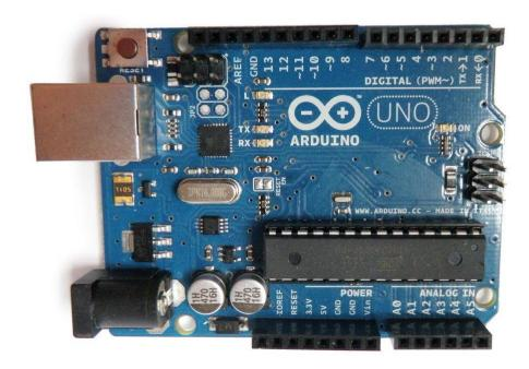
Some people think of the entire Arduino board as a microcontroller, but this is inaccurate. The Arduino board actually is a specially designed circuit board for programming and prototyping with Atmel microcontrollers.
