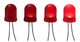
As mentioned earlier, the Arduino has a number of built in special functions. One of these special functions is pulse width modulation, which is the way an Arduino is able to create an analog-like output.
