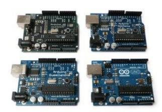
There are a number of different types of Arduinos to choose from. This is a brief overview of some of the more common types of Arduino boards you may encounter. For a full listing of currently support Arduino boards, check out the <u>Arduino</u> hardware page.
