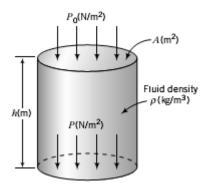
**For Example**, suppose that the cylinder of fluid in Figure above is a column of mercury that has an area of 1 cm<sup>2</sup> and is 50 cm high. The density of the Hg is 13.55 g/cm<sup>3</sup>. Thus, the force exerted by the mercury alone on the 1 cm<sup>2</sup> section of the bottom plate by the column of mercury is:
