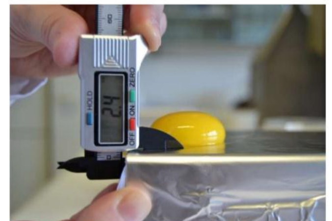
Step 6 : Measure the height (h) of the support
