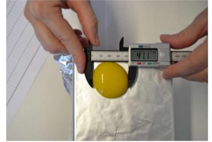
Step 3 : Measure the diameter (D1) of the yolk
