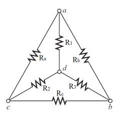
Example Calculate the total resistance of the circuit shown below
